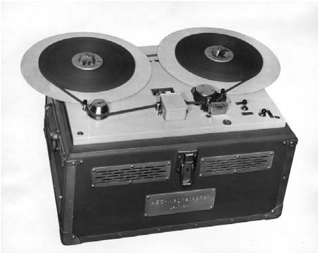
The playback device Magnetophon K 5, drive. The mechanics are largely the same as those of the Magnetophon K 4. The small shielding housing (centre front) covers the playback head. The accompanying documents refer to this instrument as the "Führergerät".
