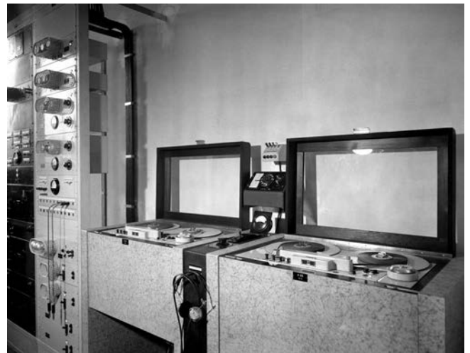
Magnetofon system R 122 (the RRG designation). Amplifiers and power supplies for the two R 22 drives are installed in the amplifier rack on the left in the picture.
